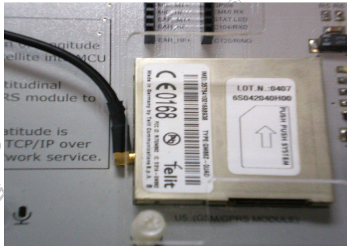
Figure E2-1-1 Connecting GSM/GPRS Module to quad-band antenna
